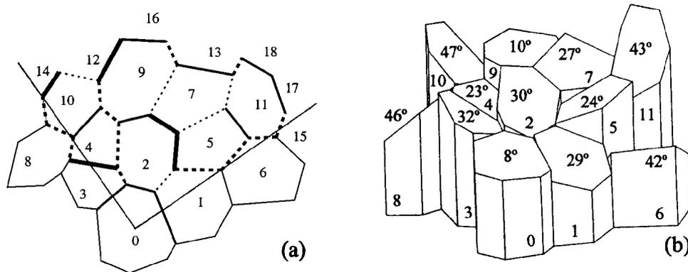
**Figure 3:** (a) Cross-section of the model. The crack propagates sequentially from grain 0 into grains 1 to 18. The grain boundary failure mechanisms are shown using the notation introduced in figure 2. (b) Perspective view of the fracture surface across the twelve complete prismatic grains of the model.
