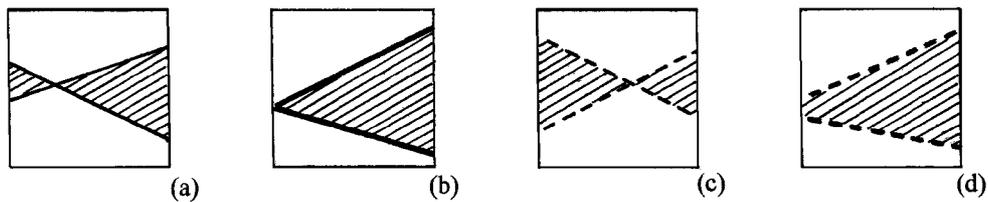
**Figure 2:** The four grain boundary failure mechanisms, arising from a cleavage crack propagating either (a) across the face of a grain or (b) from the edge of a grain or (c) meeting and (d) not meeting an approaching cleavage crack in a neighbouring grain.
