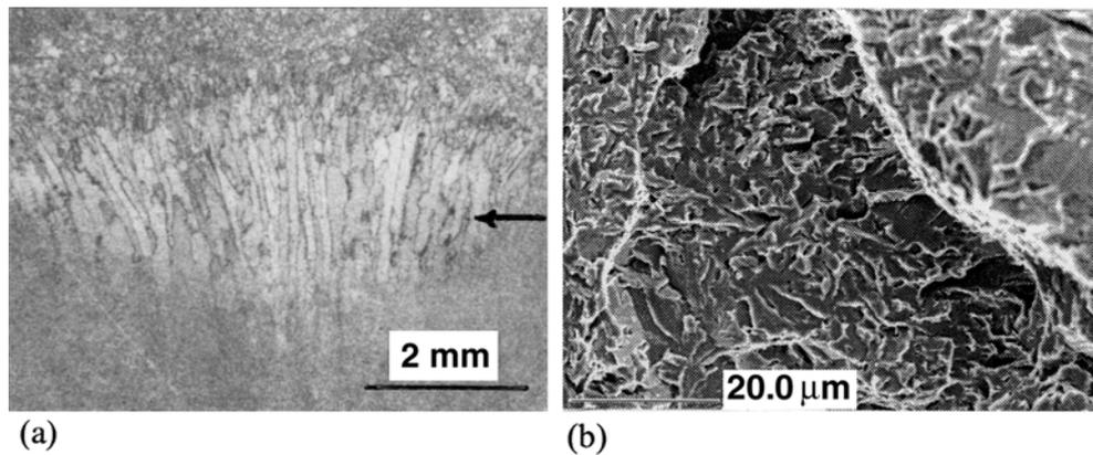
**Figure 4:** (a) Optical micrograph showing the columnar grains in a weld bead; the arrow indicates the fracture path. (b) Scanning electron fractograph of the corresponding fracture surface.
