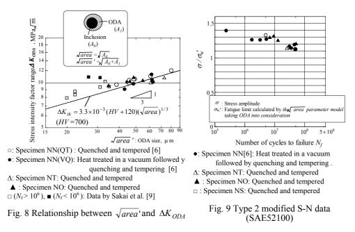
(1) The inclusion size at fracture origin is sufficiently larger than critical size of inclusion under the applied stress.
