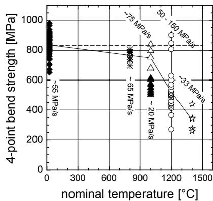
**Fig. 5:** Temperature dependence of 4-point bend strength. The mean loading rate for the test series is indicated in the diagram. Tests were performed by five different labs.
