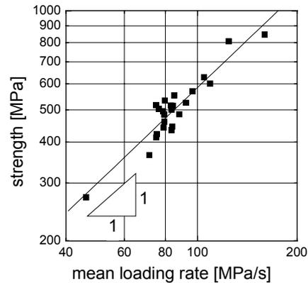
**Fig. 6:** Influence of loading rate on fracture strength at 1200°C, constant load rate tests are not shown in this diagram.
