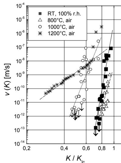
**Fig. 8:**  $v$ - $K$ -curves for four different temperatures. Arrows indicate suspended tests. The crack geometry factor was assumed to be  $Y = 1,3$ .
