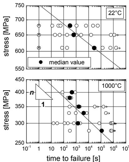
**Fig. 7:** Lifetime of the ESIS silicon nitride in deionized water at 22°C and in ambient air at 1000°C. × denotes spontaneous failure, → denotes suspended tests.
