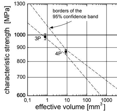
**Fig. 2:** Dependence of the characteristic strength on the effective volume.
