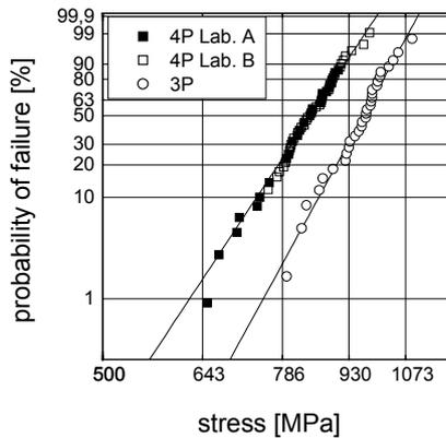
**Fig. 1:** Weibulldiagram of 3 point bend tests and 4-point bend tests.
