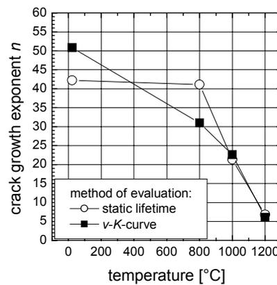
**Fig. 9:** Comparison of values for the crack growth exponent  $n$ : comparison of two different evaluation methods and temperature dependence.
