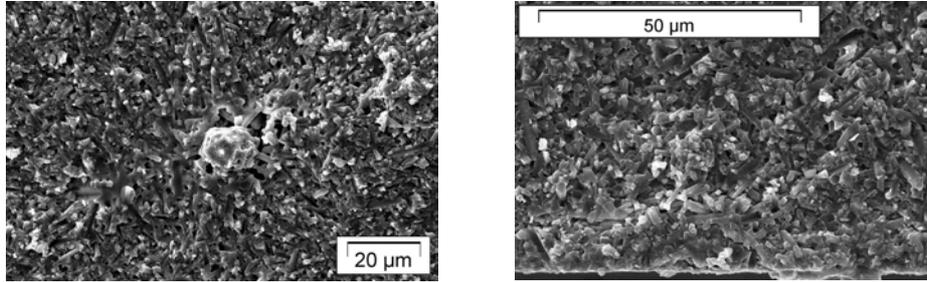
**Fig. 3:** Fracture origins in bend specimens: a) volume defect: Iron-inclusion, b) defect close to surface: insufficiently compacted region.
