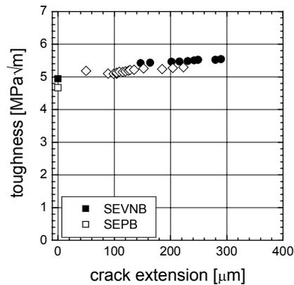
**Fig. 4:**  $K_{Ic,0}$  values measured with the SEVNB and the SEPBB technique and R-Curve.
