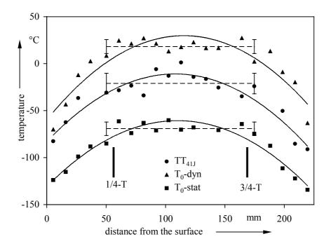
Fig. 2 Effect of specimen location on the ductile-brittle transition temperature determined by dynamic  $(T_o^{dyn})$  and static  $(T_o^{stat})$  master curve procedure and Charpy-V impact tests  $(TT_{41J})$
