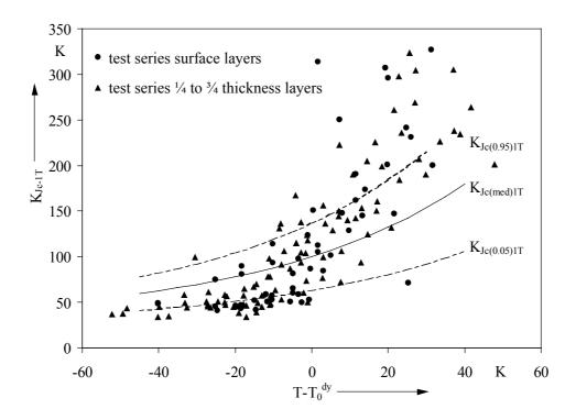
Fig. 1 Thickness corrected dynamic fracture toughness K<sub>Jc-1T</sub> for material investigated
