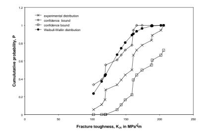
Fig. 4 Comparison of the experimental distribution and the Weibull-Wallin distribution for  $T_{Test} = 16,9$  °C, dynamic loading
