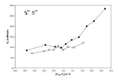
Fig. 5 Temperature dependence of the Weibull distribution normalization fracture toughness,  $K_o$  for dynamic and static loading
