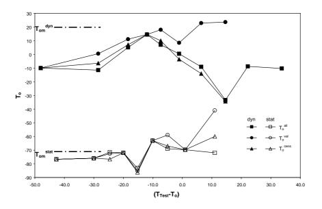
Fig. 3 Effect of the test temperature on  $T_o$  under static ( $T_o^{stat}$ ) or dynamic ( $T_o^{dyn}$ ) loading using all values measured ( $T^{all}$ ), valid values ( $T^{val}$ ) or valid and censored values ( $T^{cens}$ )
