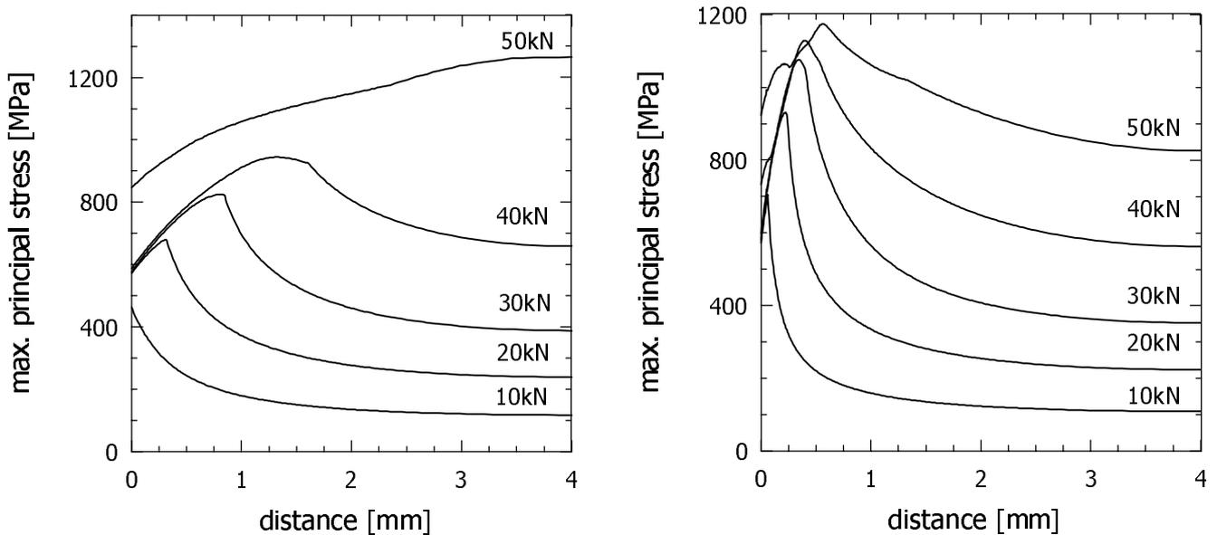
**Figure 2:** Stress distribution ahead of tip, U notch = 1 and 0.2mm
