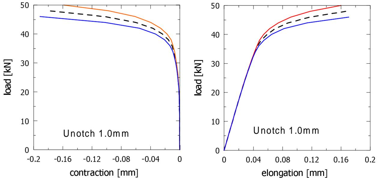
**Figure 3:** Elongation and contraction for U notch 1mm, the mean value is received from FEM, outer values correspond to the maximum and minimum of the fracture force
