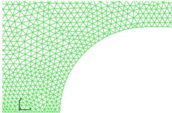
**Figure 1:** Example of a FE mesh-detail for the notched specimen  $U= 0.7. \text{ mm}$
