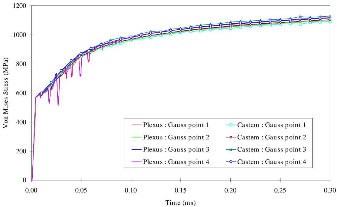
Figure 2 : Comparison between dynamic and quasi-Static 2D plane strain FE simulations of Sub-Size Charpy at -90°C.
