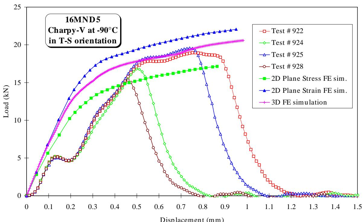
Figure 4 : Comparison of experimental and simulated (2D and 3D) load versus displacement curves for Charpy-V specimen at -90°C.
