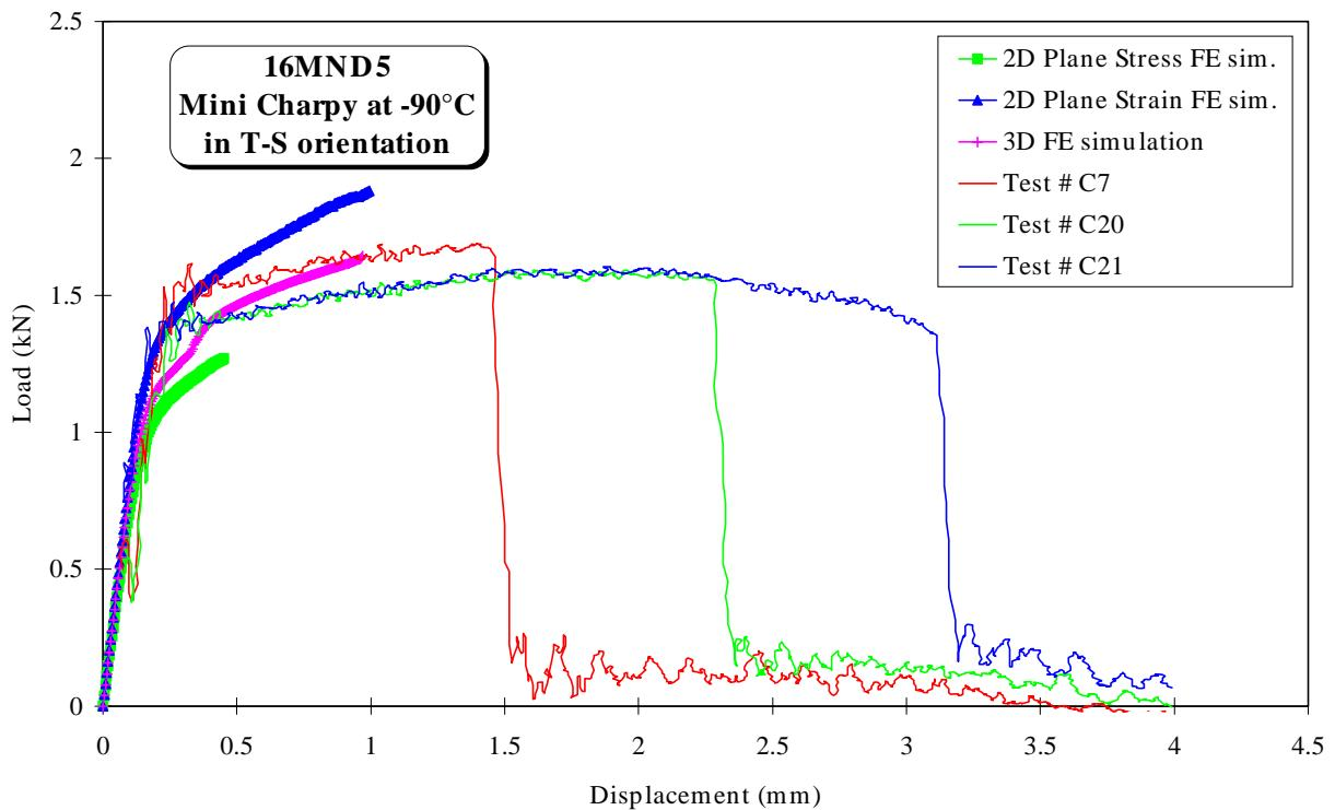
**Figure 5 :** Comparison of experimental and simulated (2D and 3D) load versus displacement curves for Sub-Size Charpy specimen at -90°C.
