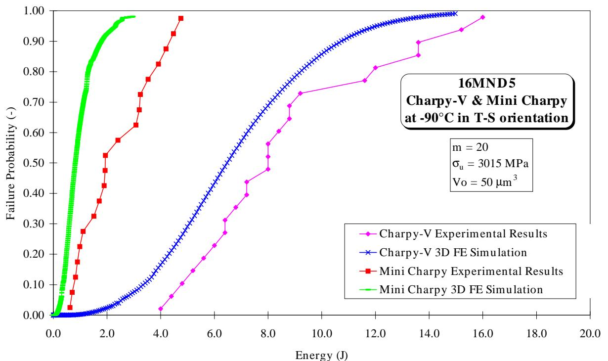
**Figure 6:** Experimental and calculated cleavage failure probability for Charpy-V and Sub-Size Charpy.
