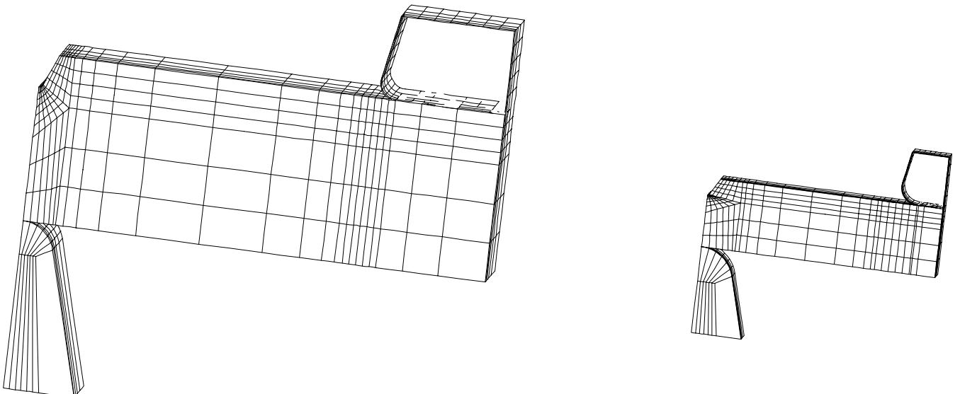
Figure 1 : 3D meshes for Charpy-V and Sub-size Charpy specimens.
