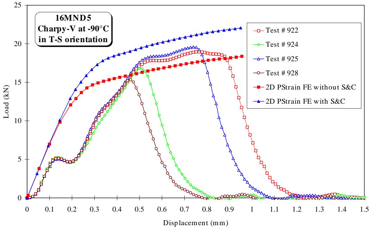
Figure 3 : Influence of strain rate on the global mechanical response for Charpy-V at -90°C.
