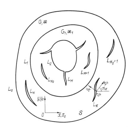
Figure 1 Two-component curvilinear ring with internal and edge cracks
