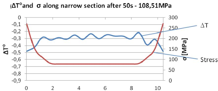
Figure 14: Temperature and axial stress along the narrow section of the specimen at 108.51 MPa.
