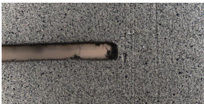
Figure 10: Initial crack in the speckled specimen (visible).
