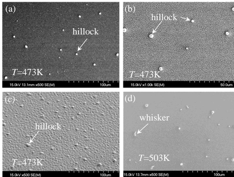
Fig. 6 Surface morphologies of annealed Sn films
