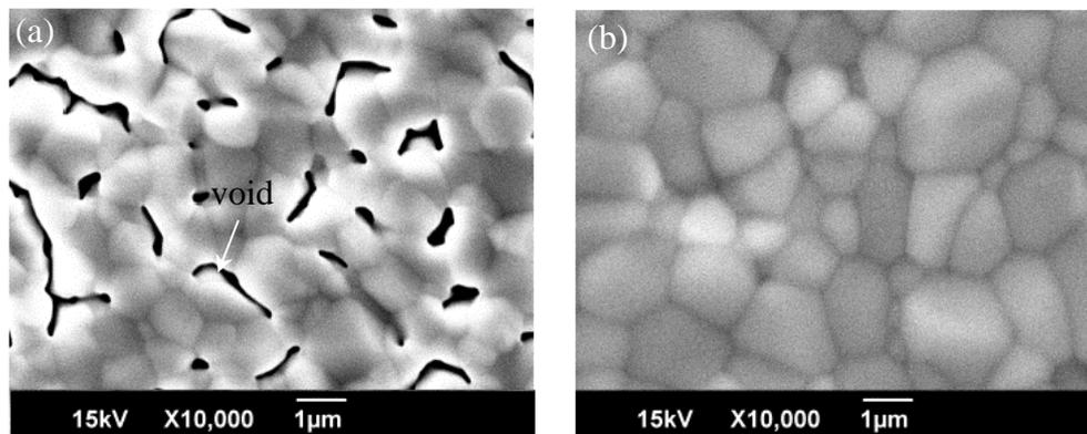
Fig. 5 Surface morphologies of Sn films with clear grains
