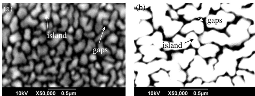
Fig. 3 Surface morphologies of Sn films with isolated island structure
