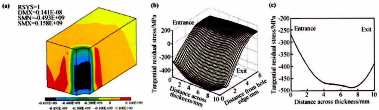
Fig.2 Tangential residual stress distribution of hole cold expanded 7050-T7451 aluminum alloy in
