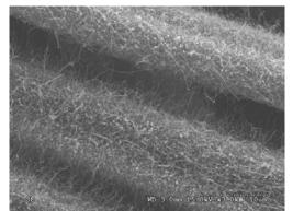
Figure 1. SEM image of a hybrid fiber with CNTs [15]
