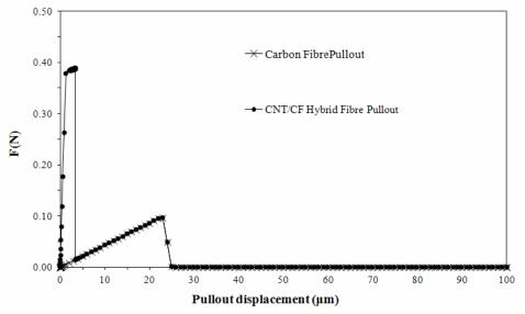
Figure 6. Comparison between the single carbon fibre pullout and the single CNT/CF hybrid fibre completed pullout curve.
