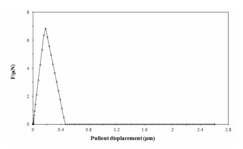
Figure 5. FE simulation for single CNT pullout curve
