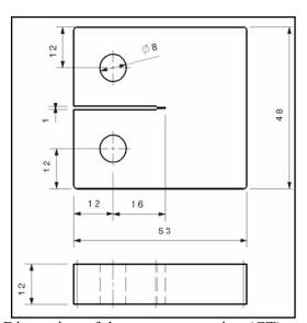
Fig.1 Dimension of the compact tension (CT) specimen.
