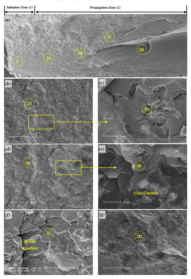
**Fig. 6** SEM micrographs of the fracture surface of UPE-3 wt. % clay nanocomposites ruptured at room temperature showing initiation and different crack propagation zones.
