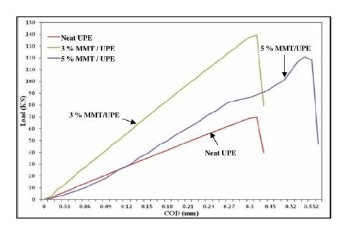
Fig. 3 Typical load vs. crack opening displacement (COD) curves.
