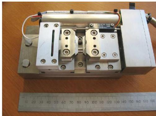
Fig. 3 Compression tester applied in micro-scale mechanical testing.
