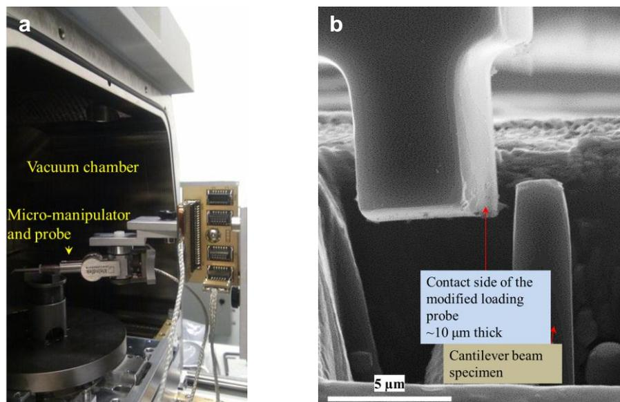
Fig. 5 (a) Installation of the FMS into the dualbeam FIB vacuum chamber. Side-view showing the FMS in the middle of the stage (b) SEM image showing loading the micro-cantilever specimen.
