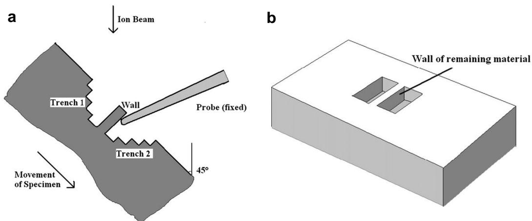
Fig. 4 (a) Schematic of the trench-probe method for applying a force to a prepared wall of material  $35\ \mu\text{m}$  long within the FIB; (b) the thin wall of residual materials created between the two trenches.
