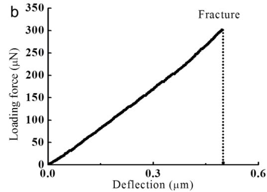
Fig. 10 A specimen created within APS-TBC. (a) Dimensions and a pre-existing flaw on the side of the cantilever with a size of  $\sim 0.1 \mu\text{m}$  as shown in insert. (b) Force-deflection curve. (c) Microstructure, dimensions of the fractured surface and the area which was in contact with the top half of the cantilever.
