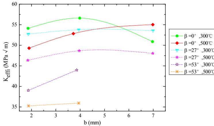
Figure 5: Results of  $K_{effi}$  versus thickness  $b$  and loading angles  $\beta$  at high temperatures (reproduced from Ref. [25])
