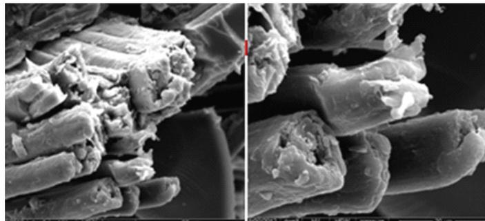
Figure 2. SEM micrographs of composites after tensile failure
