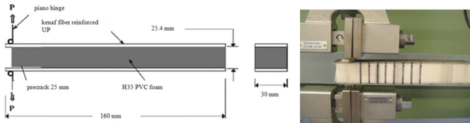
Figure 5. The dimension of double cantilever beam specimens and experiment set-up
