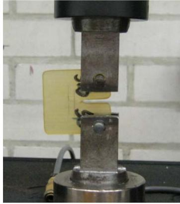
Figure 2. Quasi-static testing of CT specimen with the loading fixture
