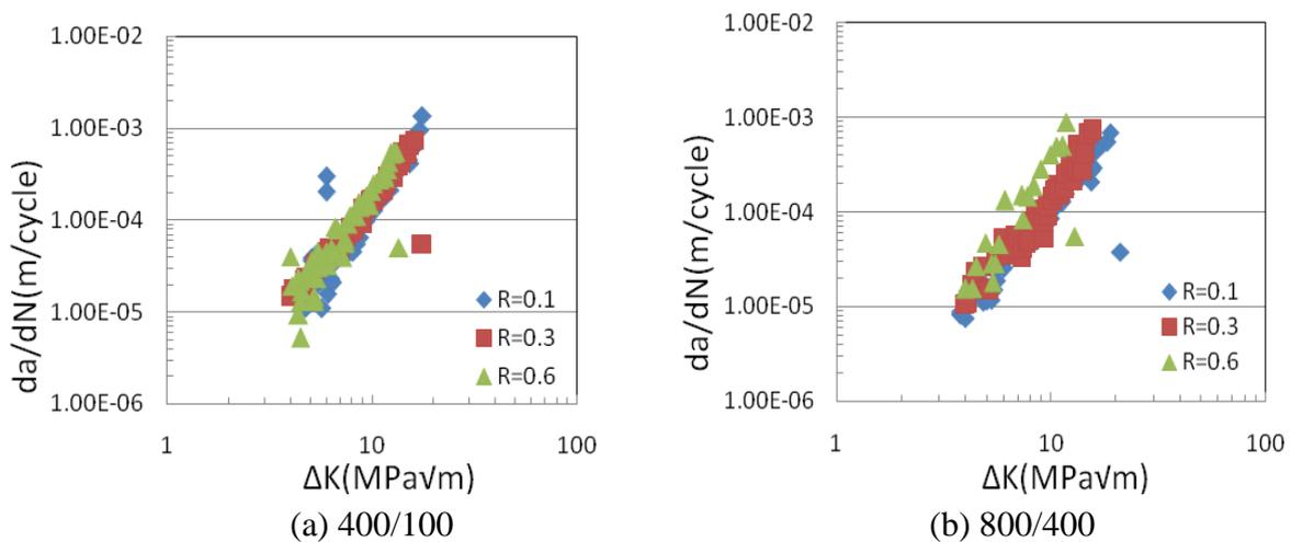
Fig.2 Crack growth rates at R=0.1, 0.3, 0.6
