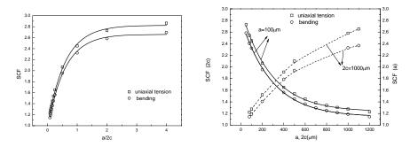
Fig. 4 SCF variation with a/2c Figure. Fig.5 SCF variation with 2c and a
