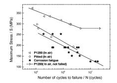
Fig. 2. S-N data for air and artificial seawater environments.
