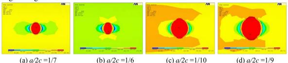
Fig. 3.The maximum stress distribution at various aspect ratios under tension (a), (b) and bending (c), (d). Cracks initiate from the point where the stress concentration is highest. Then the corrosion pit transfers to crack when the stress intensity factor for the equivalent surface crack growth for the pit reaches the threshold stress intensity factor for the fatigue crack growth, and the corrosion fatigue crack growth rate exceeds the pit growth rate.
