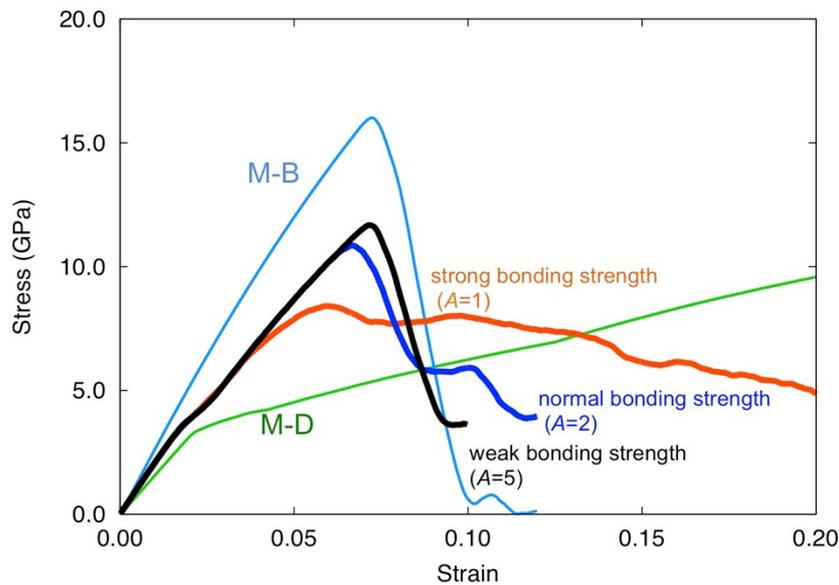
Figure 3. Stress–strain curves of multilayered composites with different interface strengths.
