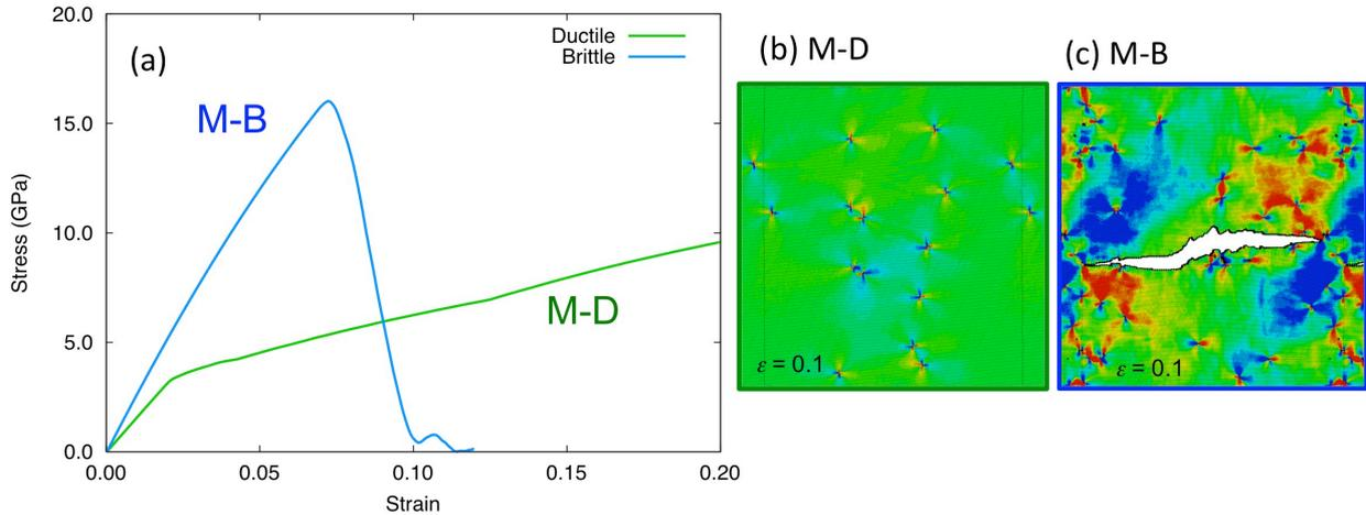
Figure 1. Stress–strain curves of virtual materials with ductile (M-D) and brittle (M-B) properties. (b) and (c) show the shear stress distributions of the single-phase models under tensile loading.
