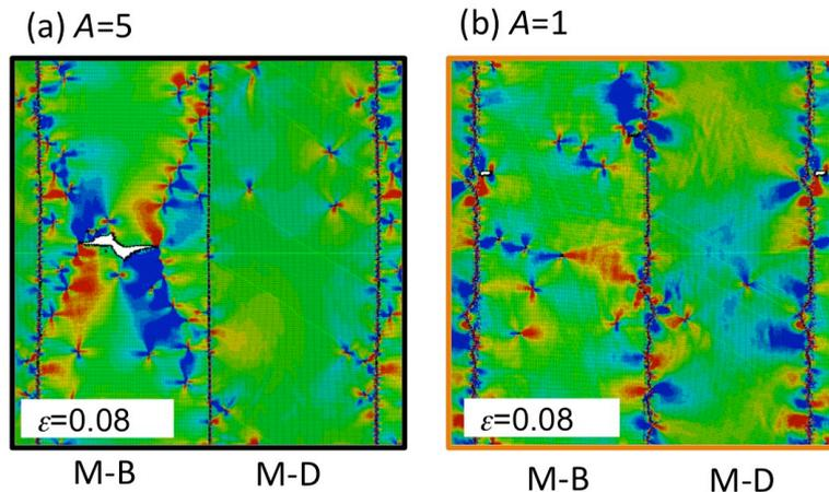
Figure 4. Plastic deformation phenomena around the interface with different mechanical properties.
