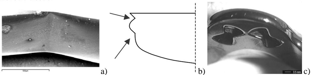
Figure 6 – a) Scratches on the leaflet near the pivots and b) their position; c) scratches inside the hinges
