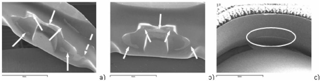
Figure 8 – Detachments of the PyC coating in the two hinges (in and out, a, b respectively) and in the housing (c).
