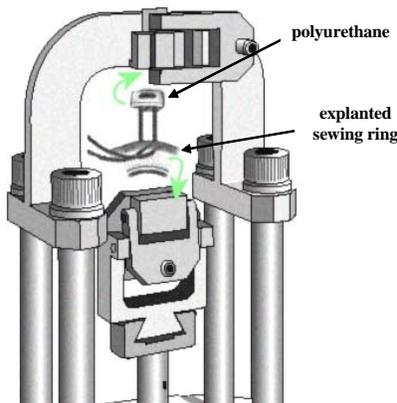
Figure 2 - Scheme of the DMA apparatus for test on suture rings
