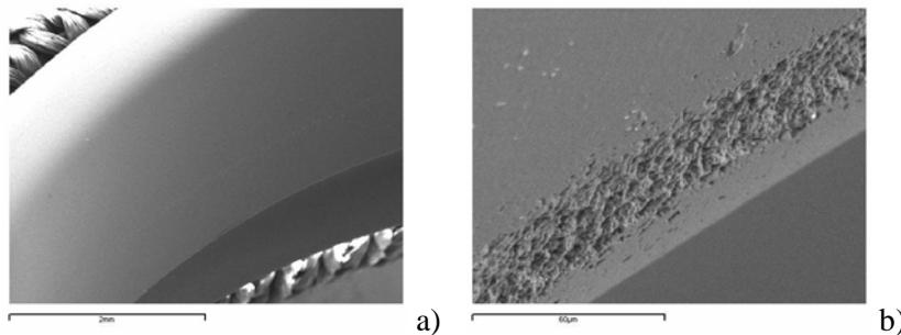
Figure 11 – Scratch due to impact wear in the housing (a), and porous surface of the scratch
