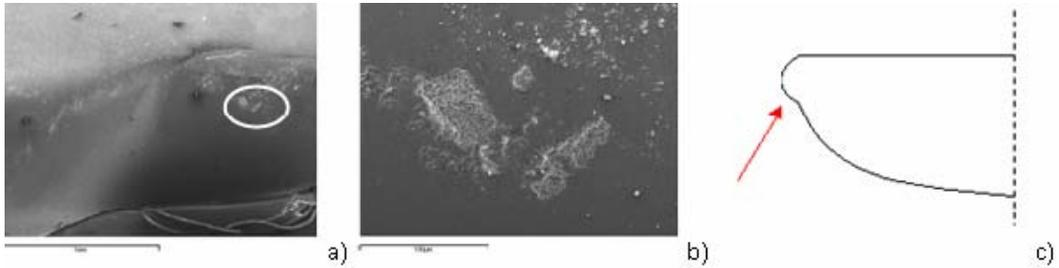
Figure 9 – Porosity of the pivots surface (a), same surface at higher magnification, the porosity is more evident (b), position on the leaflet (c).
