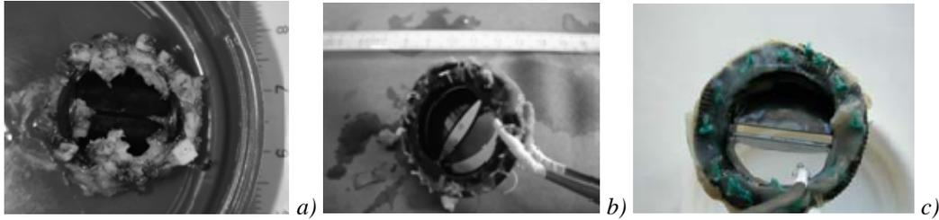
Figure 5 – Pannus on the suture ring, the correct motion of the two leaflets is obstructed: a) St Jude valve #23; b) Sorin Bicarbon #57; c) Carbomedics #36
