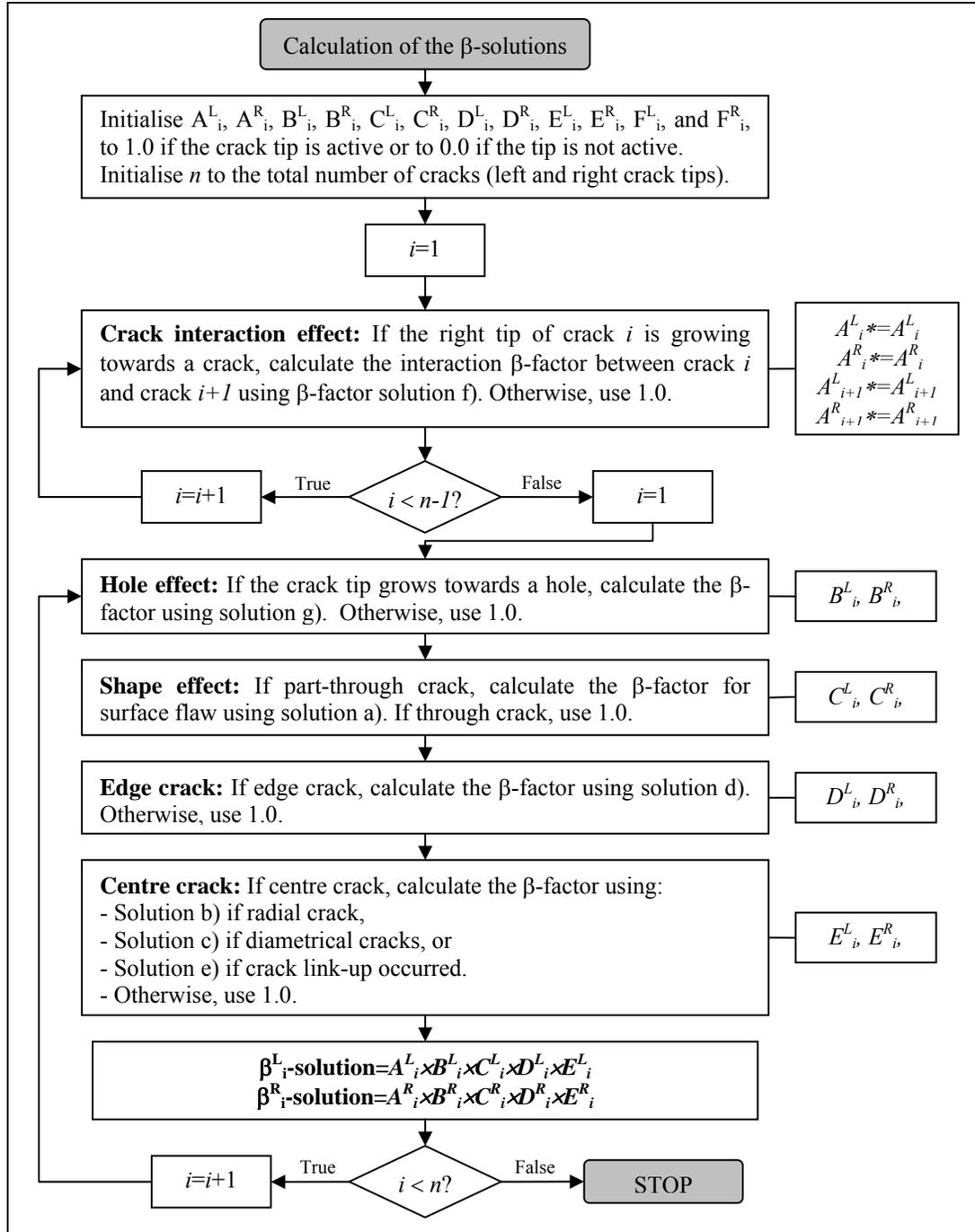
Figure 2. Generic  $\beta$ -solution compounding methodology for MSD problems.
