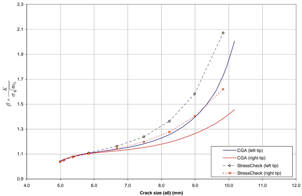
Figure 6. Comparison between the second crack ( $a_{21} / a_{22}$ )  $\beta$ -solutions obtained using NRC's CGA software and StressCheck finite element analyses.
