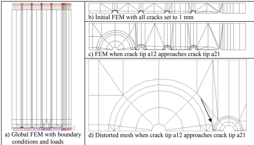
Figure 7. StressCheck finite element model.
