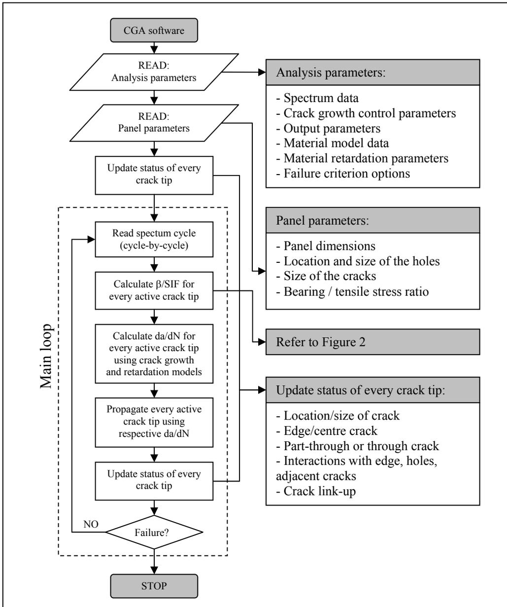
Figure 3. MSD crack growth analysis procedure.
