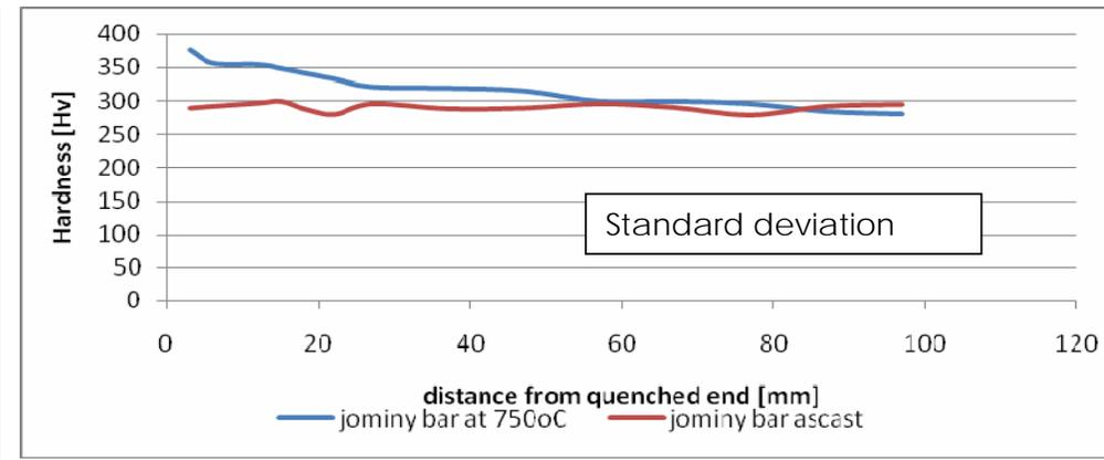
**Fig 4** Hardness profile of jominy bar at 750°C
