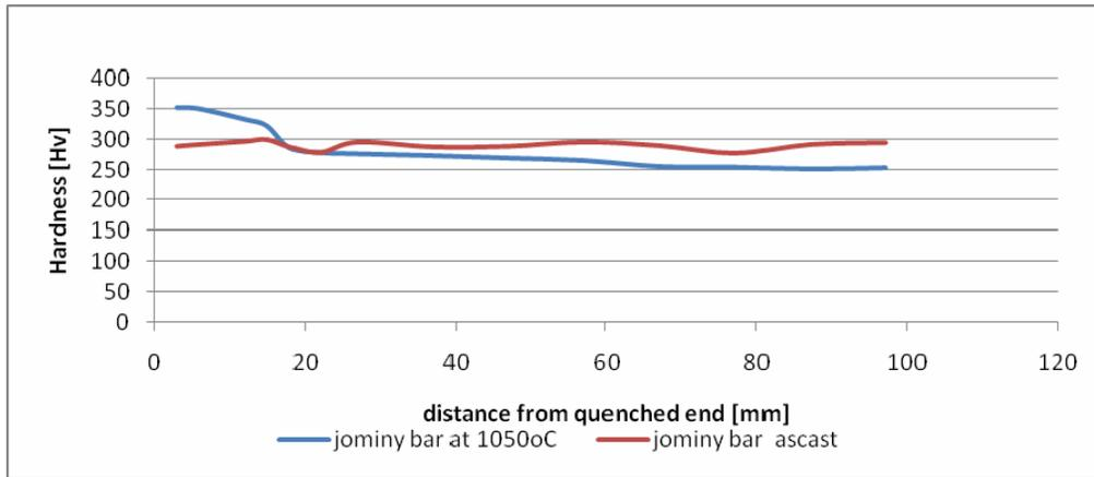
**Fig 5** Hardness profile of jominy bar at 1050°C
