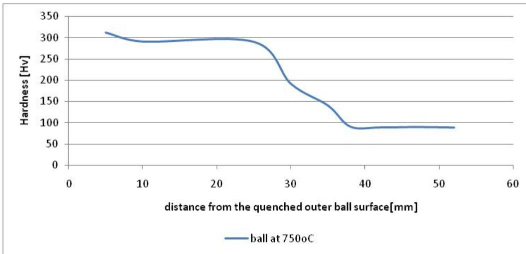
**Fig 7** Hardness for 104mm diameter ball water quenched from 750°C
