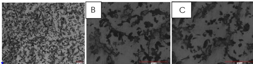
**Fig 1** Micrographs of manganese steel at 750°C: (a) Quenched jominy sample surface; (b) 50 mm from quenched end; (c) 100 mm from quenched end
