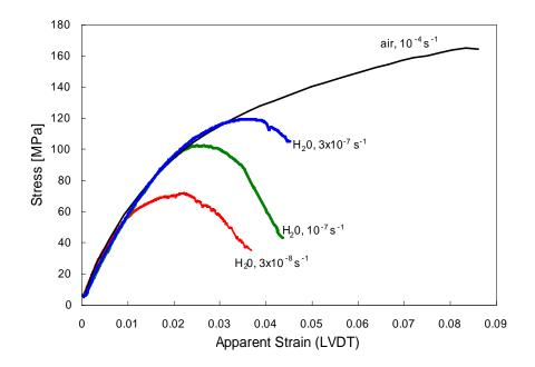
Fig. 1: Stress vs. apparent strain curves measured in CERT tests at various strain rates on tensile specimens of the Mg alloy AZ91 in distilled water and in laboratory air.
