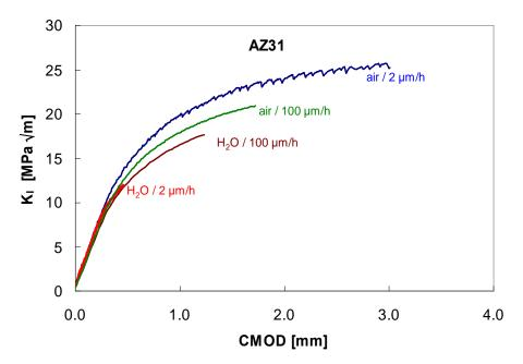
Fig. 3: Curves of the stress intensity factor, K<sub>I</sub>, vs. crack mouth opening displacement, CMOD, measured in tests on pre-cracked C(T) specimens of the Mg alloy AZ31 at two extension rates in distilled water and in laboratory air and plotted up to the onset of cracking observed in each test.
