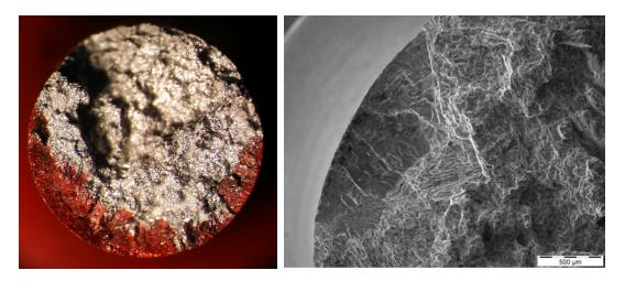
Fig. 2: Fracture surfaces of an AZ91 tensile specimens tested under constant load in distilled water, showing areas of hydrogen induced cracking; left: optical microscope, right: scanning microscope.
