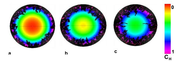
Fig. 4: Simulation of the hydrogen induced failure of a tensile specimen; the pictures show cross sections of the specimen at various stages of the failure process, the black areas indicate pits/broken fibres, the area in the centre represent uncracked ligament, and the seams around the black areas indicate different concentrations of hydrogen in the diffusion front according to the bar at the extreme right.
