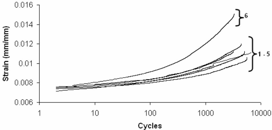
Fig. 2. Strain accumulation under dwell fatigue conditions.
