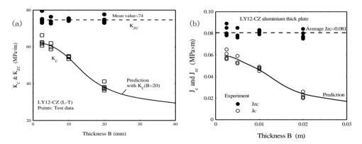
Fig. 3. Variation of two- and three- dimensional fracture toughness parameters  $K_{\rm C}$ - $K_{\rm ZC}$  (a) and  $J_{\rm C}$ - $J_{\rm ZC}$  (b) with thicknesses of test specimens.
