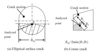
Fig.5. Definition of equivalent thickness  $B_{eq}$  for 3D cracked bodies.
