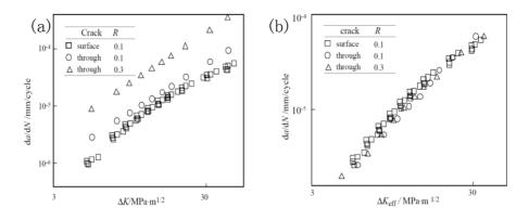
Fig.6 da/dN~ $\Delta K$  (a) and da/dN~ $\Delta K_{eff}$  (b) curves of 20CrMo steel.
