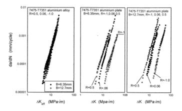
Fig. 4. Fatigue crack growth data in 7475-T7351 aluminum alloy: CCT specimens with different thicknesses.
