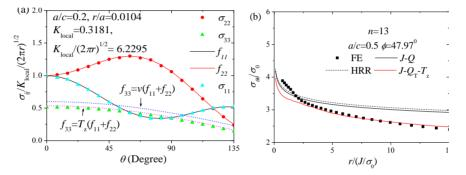
Fig. 2. (a) The elastic stress components of semi-elliptical surface crack front line at  $\phi$ =45.14 °, (b) The description of elastic-plastic stress parameters  $\sigma_{\theta\theta}/\sigma_0$  of semi-elliptical surface crack front line.
