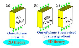
Fig. 1. Finite thickness plates under in-plane loading.
