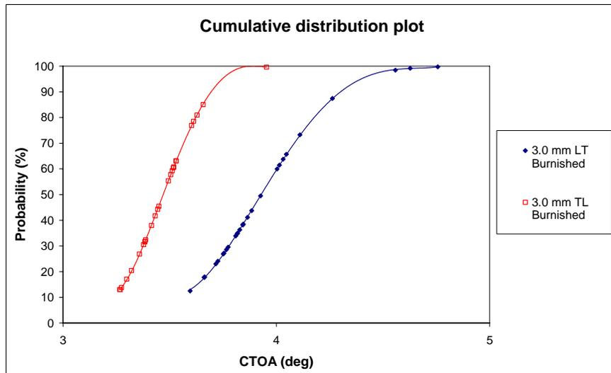
Figure 10 Cumulative probability plot for CTOA data in the steady state region.
