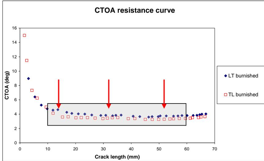
Figure 9 CTOA Resistance for both specimens, grey box indicates the steady state region and arrows denote the centre of the burnished stripes on the LT specimen.
