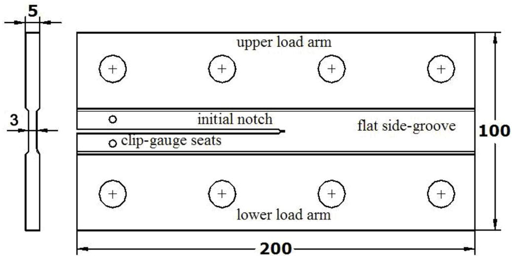
Figure 2 Dimensions of mDCB specimens used.
