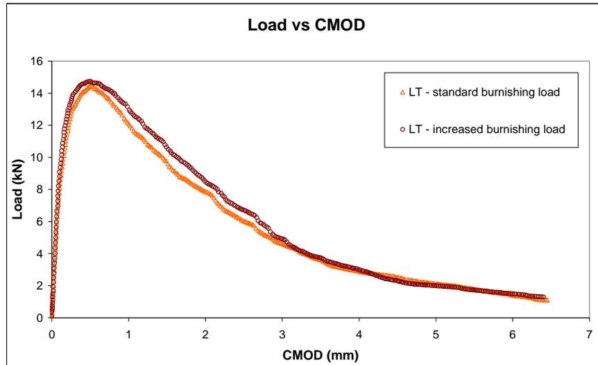
Figure 11 Preliminary data for CT specimens burnished under similar conditions.
