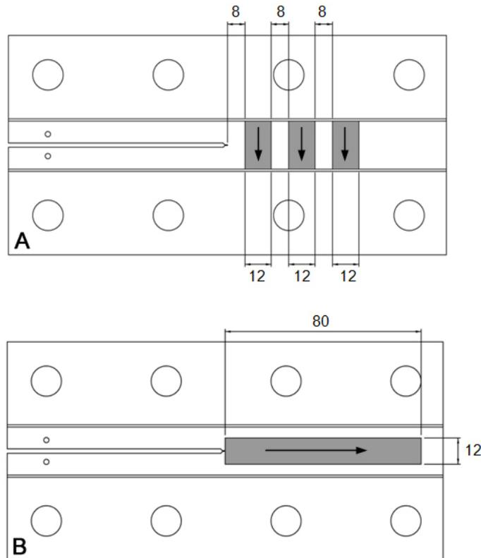
Figure 5 Burnishing regimes, grey areas indicate burnished stripes and arrows indicate the direction of burnishing. Identical regimes were applied to both sides of the specimen.
