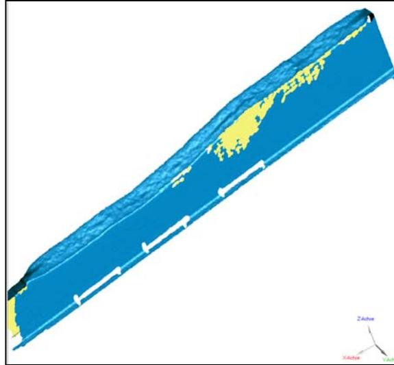
Figure 8 3D reconstruction of the fracture surface (courtesy of IVB GmbH)
