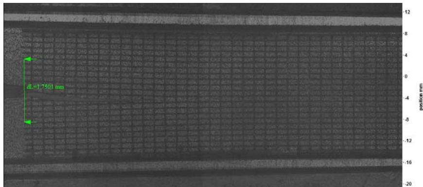
Figure 4 Showing CMOD measurement and etched grid for CTOA measurement comparison
