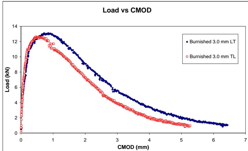
Figure 7 Load – CMOD data for both specimens.
