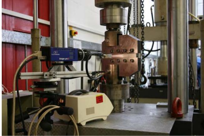
Figure 3 Experimental setup for tear tests.
