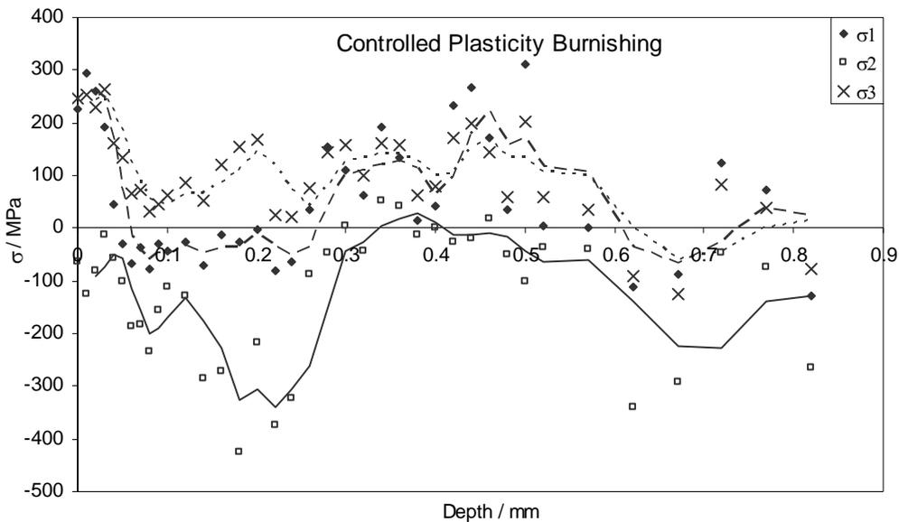
Figure 1 3D residual stress state in CPB 2024-T351
