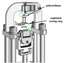
Figure 2 - Scheme of the DMA apparatus for test on suture rings
