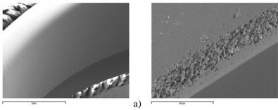
Figure 11 – Scratch due to impact wear in the housing (a), and porous surface of the scratch
