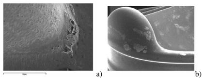
Figure 7 – Housing of valve #15 porous surface in the hinge (a); valve #23 porous areas on the outer surface of the housing and in the centre of the leaflets (b)
