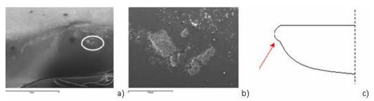
Figure 9 – Porosity of the pivots surface (a), same surface at higher magnification, the porosity is more evident (b), position on the leaflet (c).
