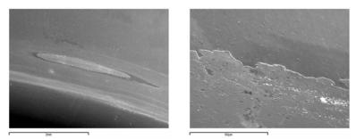
Figure 10 – Scratches and PyC coating detachment correlated to defects in the surface finishing process
