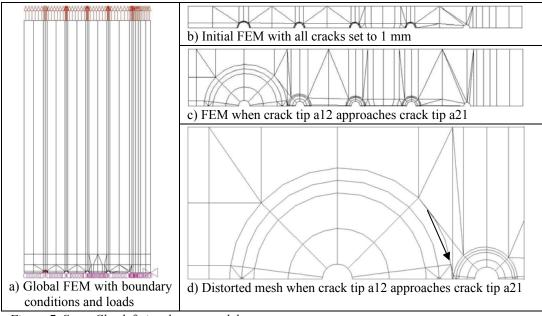
Figure 7. StressCheck finite element model.
