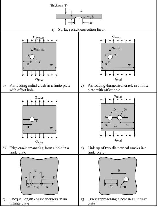
Figure 1. Schematic representation of the  $\beta$ -factors used to solve MSD problem by the principle of superposition.
