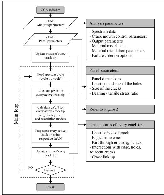
Figure 3. MSD crack growth analysis procedure.
