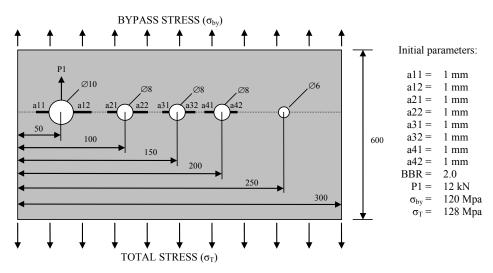
Figure 4. Parametric MSD panel case study. Dimensions are in millimetres (mm).
