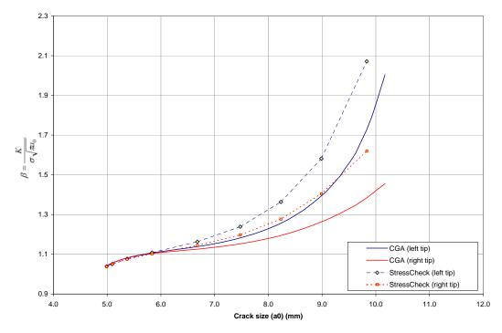
Figure 6. Comparison between the second crack  $(a_{21} / a_{22}) \beta$ -solutions obtained using NRC's CGA software and StressCheck finite element analyses.
