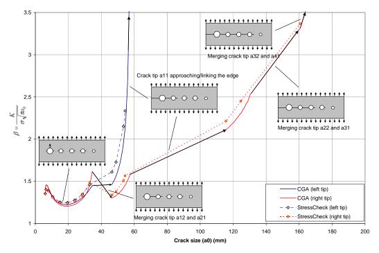
Figure 5. Comparison between the lead crack  $(a_{11} / a_{12}) \beta$ -solutions obtained using NRC's CGA software and StressCheck finite element analyses.
