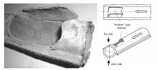
Figure 1: "Window" type fracture with schematic view of the damage.
