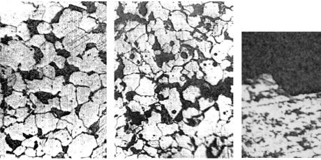
Figure 2: Ferrite - pearlite. Figure 3: Ferrite. Decarburization. Fisures. 500x
