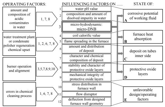
Figure 5: Summary of influencing factors for hydrogen damages of boiler evaporator tubes
