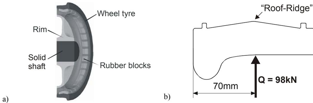
Figure 1: a) Assembly of a rubber-sprung wheel (CAD-model of a half-wheel)
