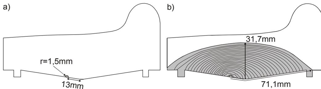
Figure 4: Numerical crack growth simulation for the ICE-wheel tyre with a diameter of 862mm and wheel contact force  $Q = 98\text{kN}$
