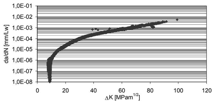
Figure 5: Crack growth rate curve for the wheel tyre material (B5)
