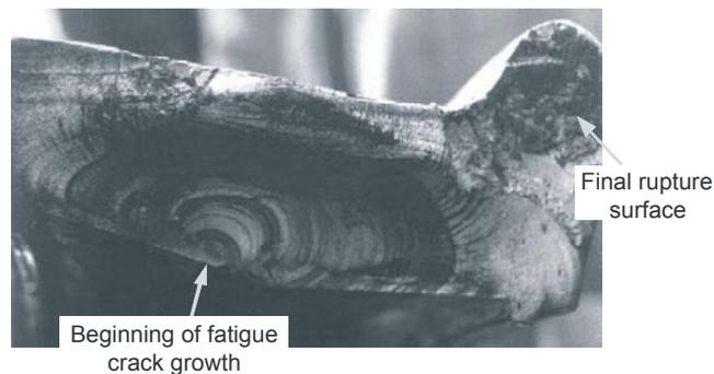
Figure 3: Fracture surface of the broken wheel tyre
