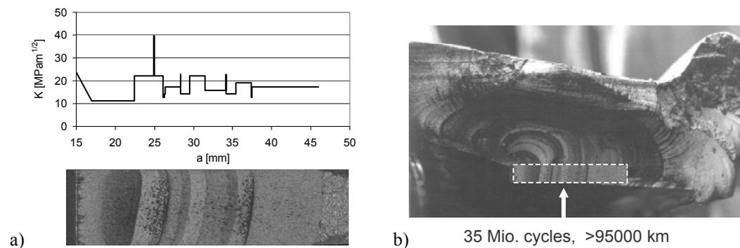
Figure 6: a) Relationship between loading and fracture surface in the experiment
