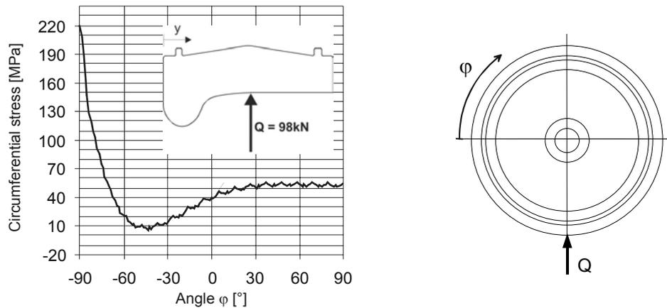
Figure 2: Circumferential stress on the inner surface of the wheel tyre at  $y=67,5\text{mm}$  (“roof-ridge”) in dependence of the angle  $\varphi$  for the loading case straightforward driving (assembly + Q-Force) for a wheel diameter of 862mm
