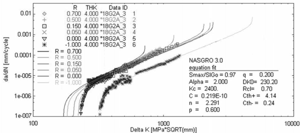
Figure 1:  $da/dN$  versus  $\Delta K$  data from the CA tests and the corresponding material parameters used in the NASGRO SY model
