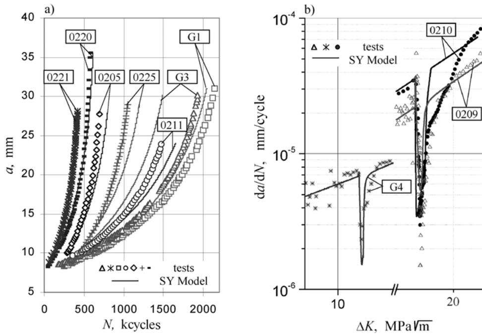
Figure 5: Comparisons between the experimental results and predictions from the SY model according to the present authors: (a) CA tests; (b) OL tests
