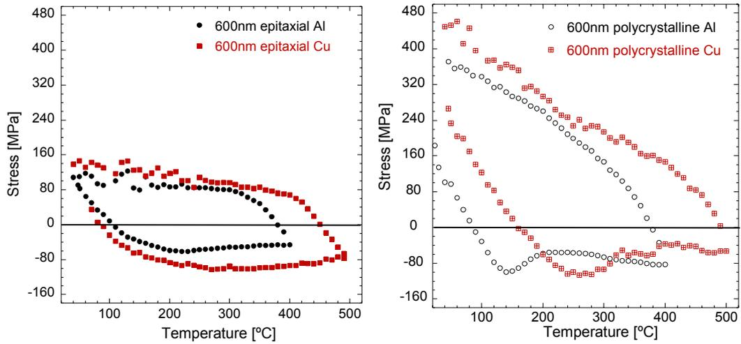
Fig. 2: Thermal stress evolution of 600nm thick (a) epitaxial and (b) polycrystalline Al and Cu films, respectively, as measured with a substrate-curvature technique [3].
