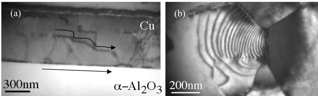
Fig. 3: (a) A threading dislocation gliding on an inclined  $\{111\}_{\text{Cu}}$  plane gets constrained between a Cu twin boundary and the film/substrate interface. The advancing dislocation is forced to deposit interfacial dislocation segments at both interfaces (see arrows) [3]. (b) Parallel glide dislocations [4] emitted from a grain boundary in a 150nm thick Cu film during cooling from 500°C to 40°C.
