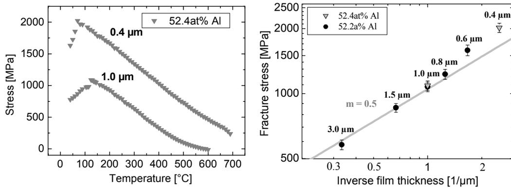
Fig. 4: (a) Stress evolution on cooling from 600 or 700°C to 40°C for Al rich NiAl films. A stress drop occurs indicating fracture [6]. (b) The measured fracture stress values of NiAl films with Al contents of 52.2 and 52.4at% are shown as a function of the inverse film thickness (double logarithmic plot). Note that the fracture stresses follow a predicted slope of 0.5 indicating that the film thickness corresponds to the critical defect size [6].
