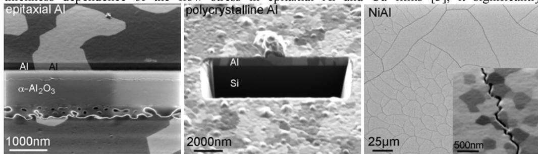
Fig. 1: FIB images of (a) a 350nm thick epitaxial (bicrystal) Al film grown on a (0001)-oriented  $\alpha$ -Al<sub>2</sub>O<sub>3</sub> single crystal [8], (b) a 1000nm thick polycrystalline Al film grown on an oxidised (001) Si substrate [3], and (c) a 1500nm thick Al rich NiAl film (52.2at% Al) on a nitrided (001) Si substrate. Note that cracks are present in the Al rich NiAl film, which run mainly along NiAl grain boundaries (see enlarged inset in (c)) [6].
