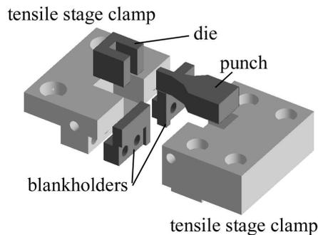
Figure 1: Exploded view of the experimental deep-draw setup.
