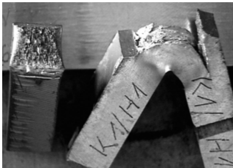
FIGURE 2: The fracture of specimens cut from the pipe being in service and subjected to the toughness tests: specimen from upper (left) and lower (right) areas of the pipe.
