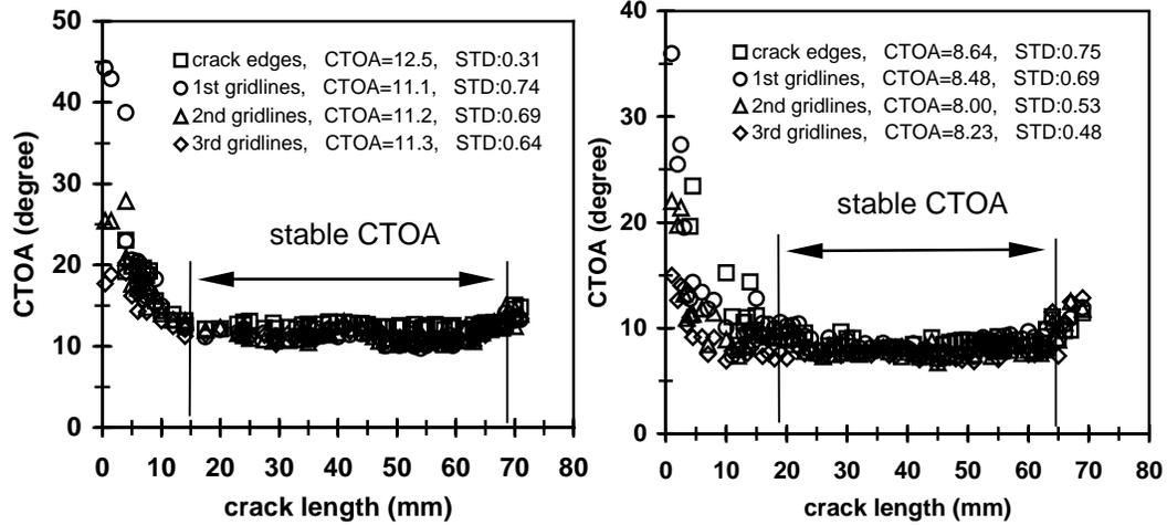
Figure 3: CTOA resistance curves for X80 (left) and X100 steel (right)
