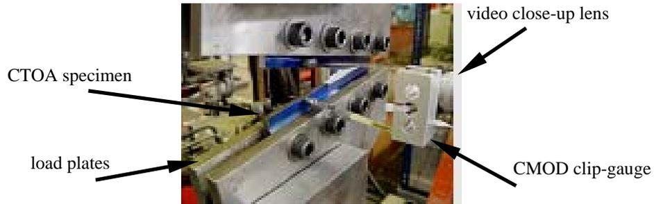
Figure 2: View of a CTOA specimen with 8mm ligament thickness after fracture
