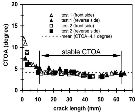
Figure 4: CTOA resistance curve for aluminium alloy
