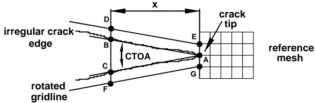
Figure 1: Determination of CTOA from the crack flanks and from the slope of the reference mesh
