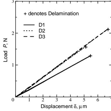
Figure 2: Load-displacement curves of PZT specimens
