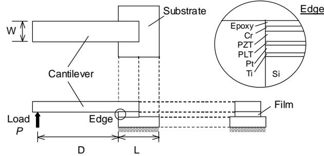
Figure 1: Schematics of PZT specimen and loading system
