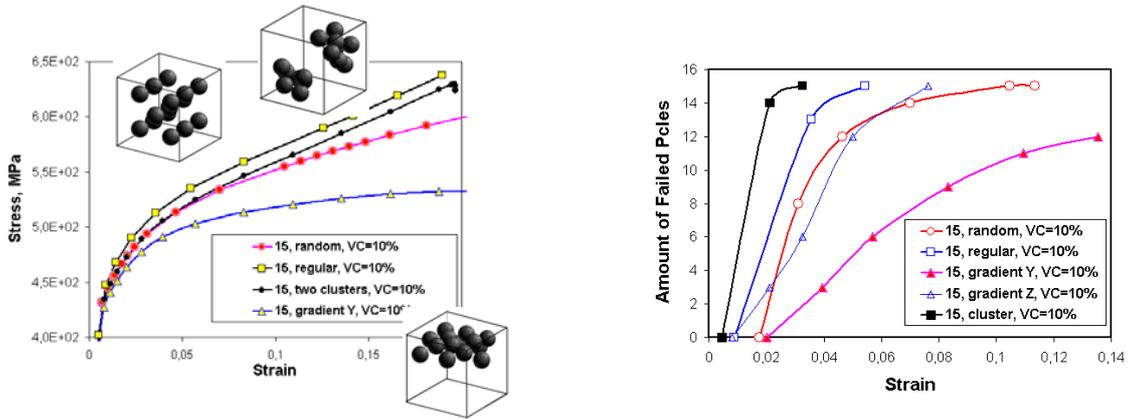
Figure 2. Tensile stress-strain curves (left) and the amount of failed particles versus the far-field applied strain curves (right) for the different arrangements of particles (random, regular, clustered and gradient).
