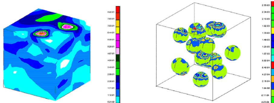
Figure 3. Distribution of equivalent plastic strains on box boundary (left), and on the particle/matrix interface in the microstructures with random particle arrangements (15 particles, VC =10%).
