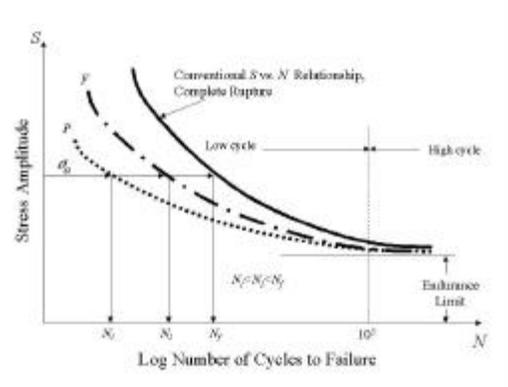
Fig. 2 Conventional representation of fatigue process
