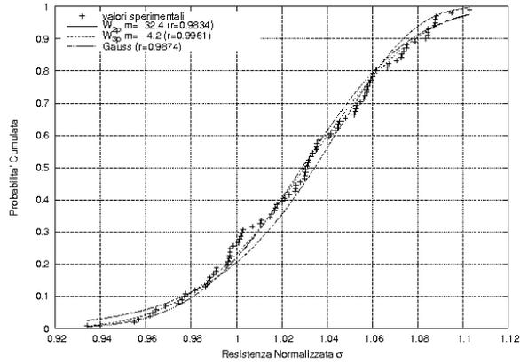
Figure 4: Probability failure vs normalized strengt ( $a_0/c_0 = 0.5$  and  $a_{sd}/c_0 = 0.3$ ).
