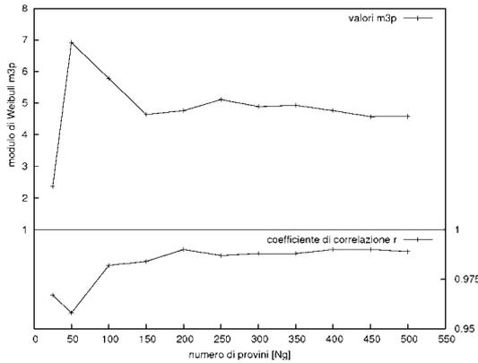
Figure 2a: Variation of the Weibull modulus with the number of specimens (three parameters distribution).
