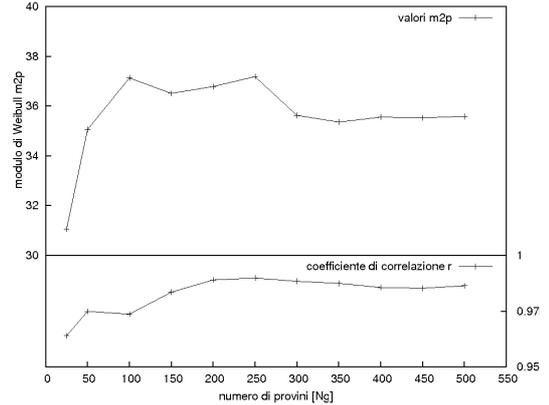
Figure 2b: Variation of the Weibull modulus with the number of specimens (two parameters distribution).
