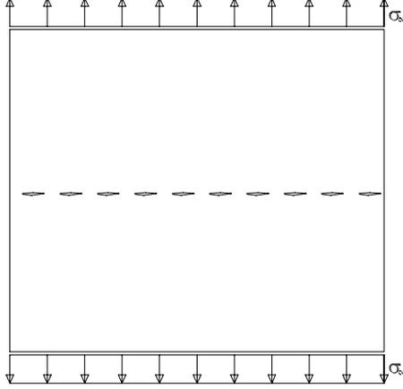
Figure 1: Infinite plate with  $N$  collinear cracks, loaded on the edges by uniform remote tension  $\sigma_\infty$ .
