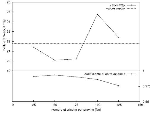
Figure 3: Variation of the Weibull modulus  $m$  with the number of cracks  $N_c$  for specimen.
