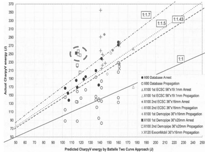
Figure 3. CSM database for X80 and X100 tests
