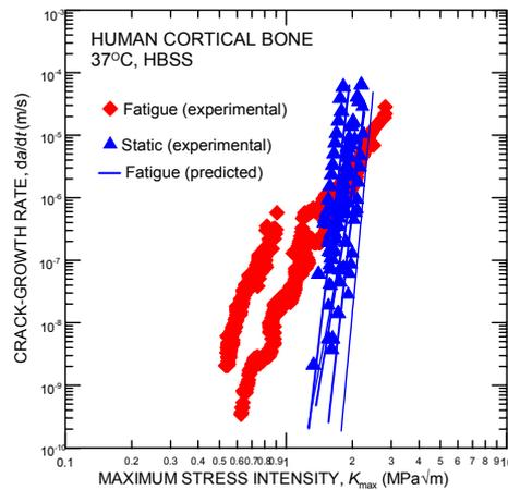
**Fig. 1:** Variation in *ex vivo* fatigue-crack growth rates,  $da/dN$  as a function of  $K_{\text{max}}$ , as compared to sustained-load cracking rates, for the proximal-distal orientation in human cortical bone.
