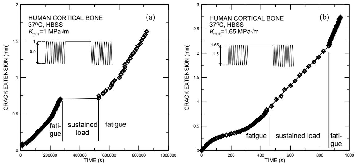
**Fig. 2:** Results of the “fatigue-sustained load-fatigue” tests at fixed  $K_{\max}$  levels, presented as plots of crack extension as a function of time, for (a)  $K_{\max} = 1 \text{ MPa}\sqrt{\text{m}}$ , (b)  $K_{\max} = 1.65 \text{ MPa}\sqrt{\text{m}}$ .
