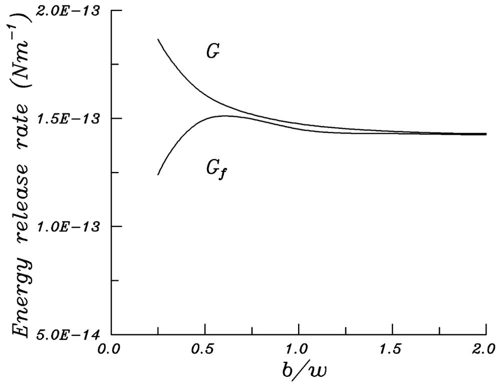
Fig. 3 Energy release rate of zirconia
