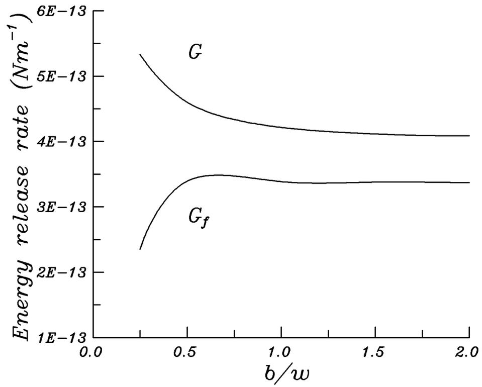
Fig. 4 Energy release rate of aluminum alloy
