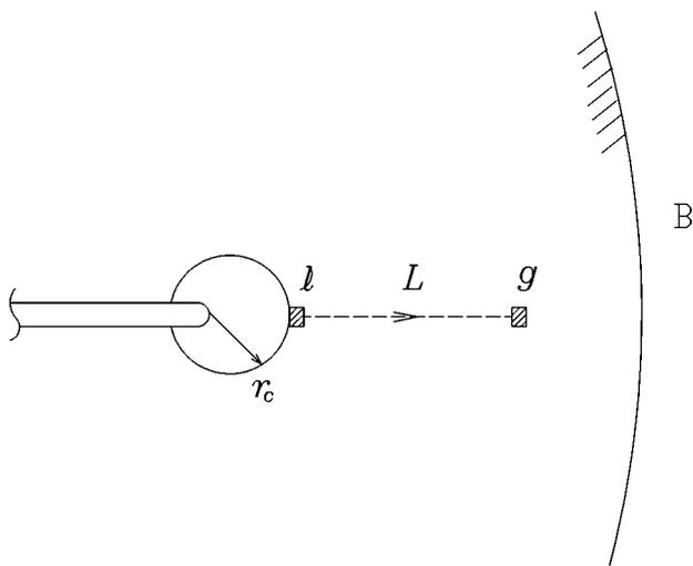
Fig. 2 Crack initiation, path, and termination
