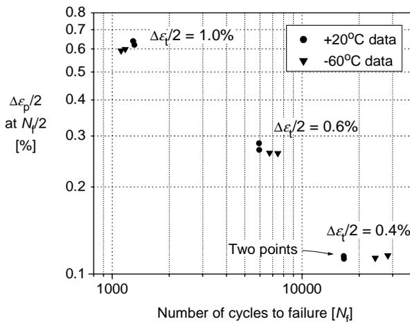
Figure 4: Fatigue life versus plastic strain amplitude
