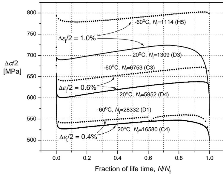
Figure 3: Stress amplitude development for tests run at both +20°C (black lines) and -60°C (dotted lines). The cycle number has been normalised to the total number of cycles to failure for each test. The kink in the sample D1 curve is caused by a temporary increase of extensometer temperature.
