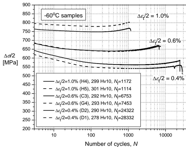
Figure 2: Stress amplitude development for tests run at  $-60^{\circ}\text{C}$
