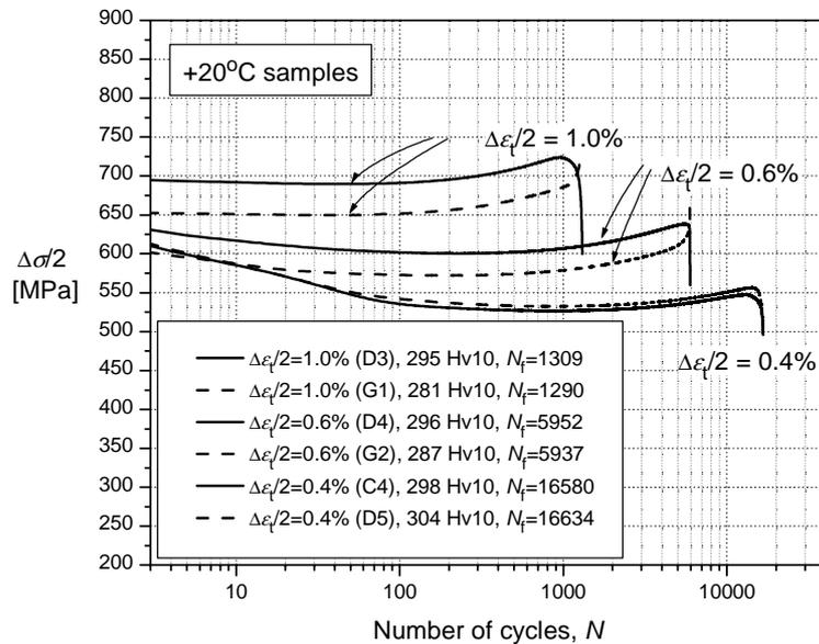
Figure 1: Stress amplitude development for tests run at + 20°C. Numbers within parantheses correspond to sample identification and are in some cases referred to in the text.
