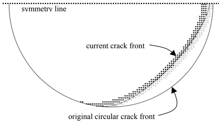
Figure 4: Predicted crack front shapes.
