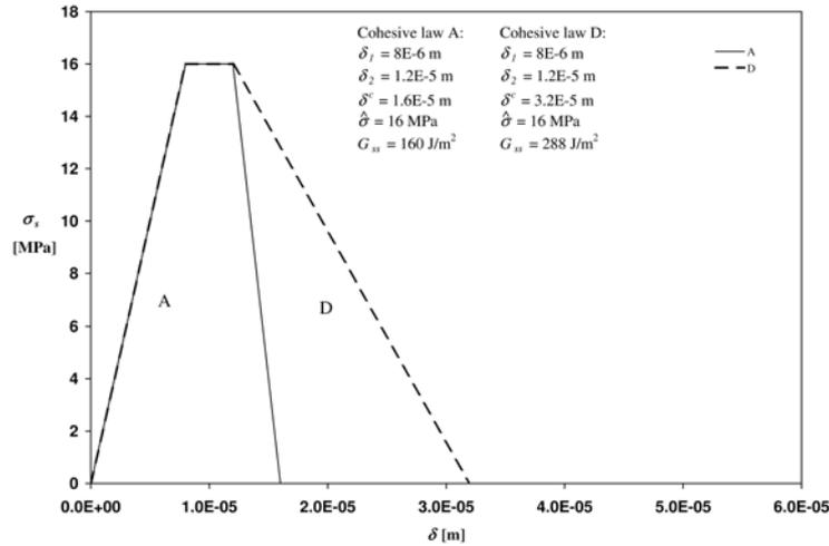
Figure 1: Two traction separation relations for the adhesive.
