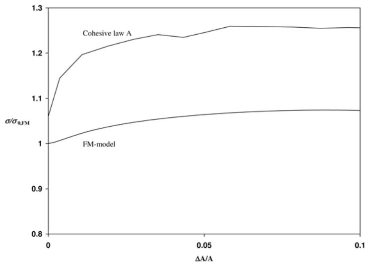
Figure 3: Relationship between applied stress and bond area change for fracture mechanical and cohesive zone model.
