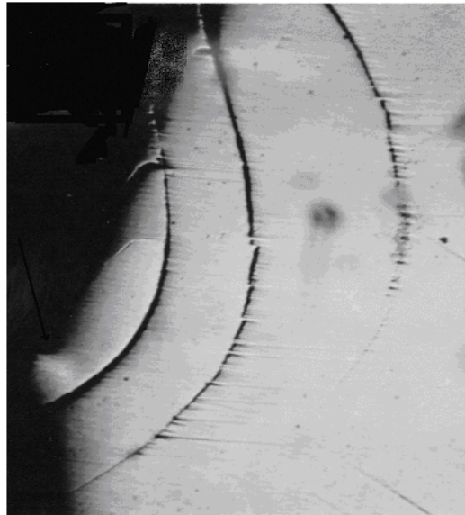
Figure 6 – Polished cross section of the broken half of a salt nitrocarburized AISI H-13 steel sample (Charpy-V notch, \rho = 0.25 mm).
