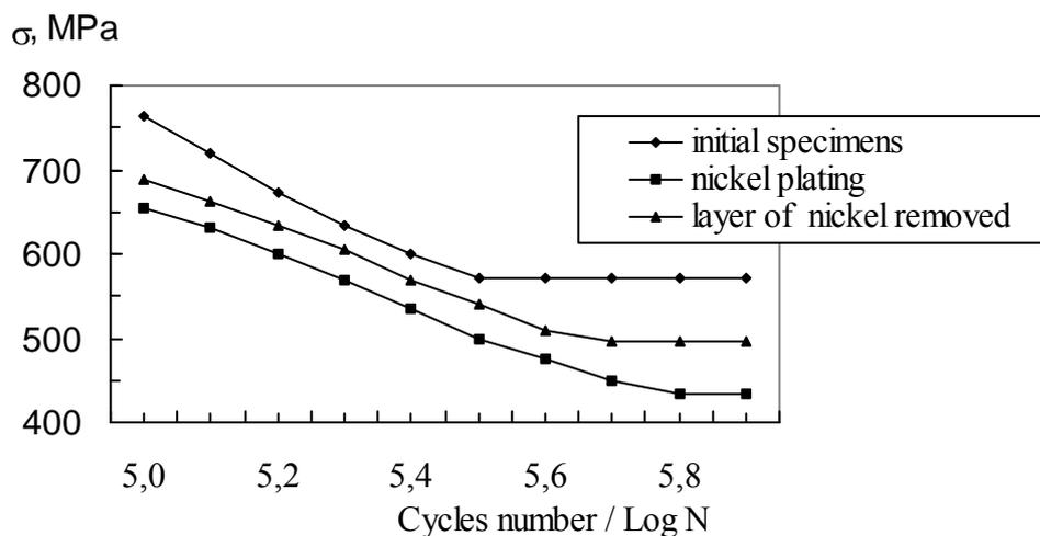
Fig.5. Curves of fatigue of specimens after electrochemical nickel plating.
