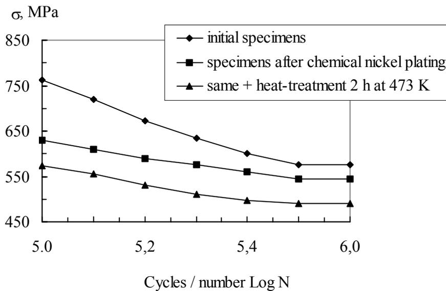
Fig. 3. Curves of fatigue of specimens after chemical nickel plating.
