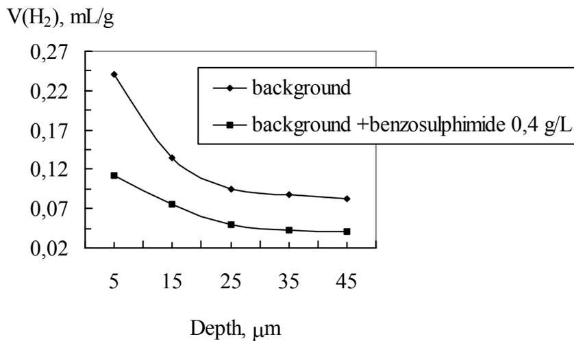
Fig. 4. Distribution of hydrogen across of steel base after electrochemical nickel plating 20  $\mu\text{m}$  thick.
