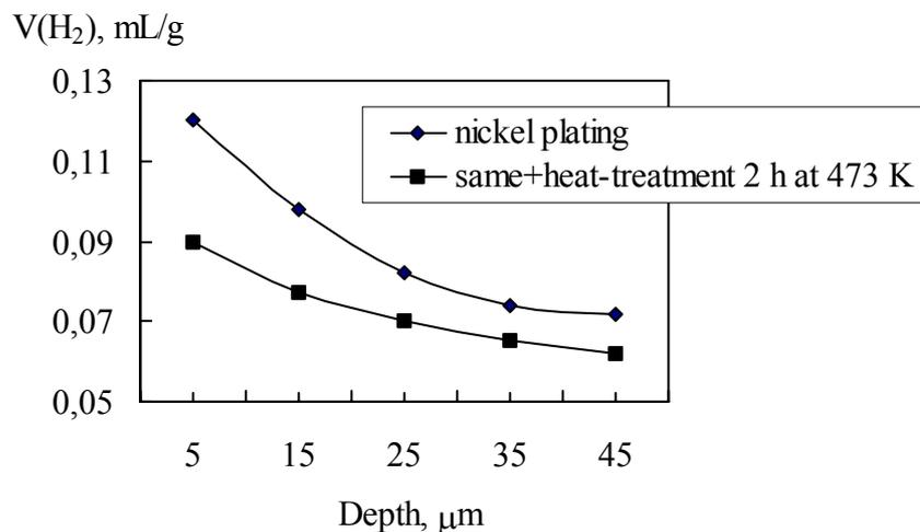
Fig.1. Distribution of hydrogen across of surface layer of the steel base after chemical nickel plating  $20 \mu\text{m}$  thick.
