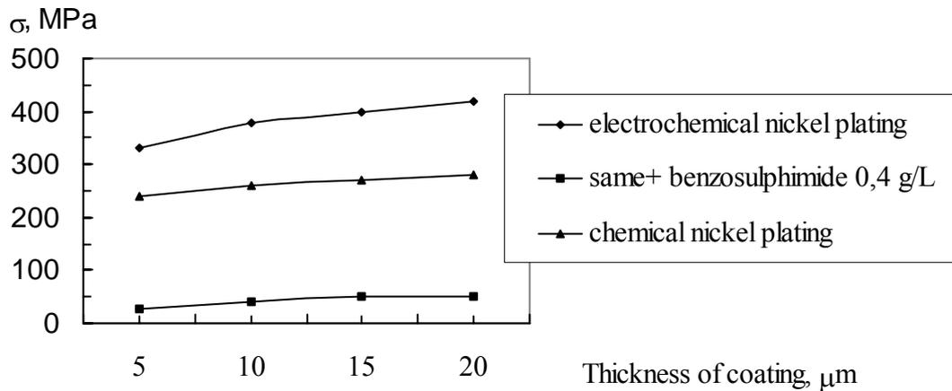
Fig. 2. Residual stresses in nickel coating.
