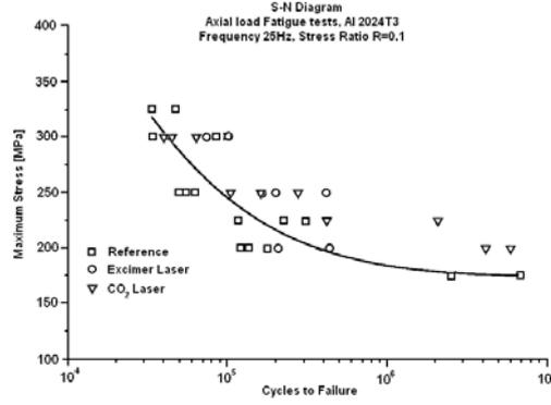
Fig. 1: *S-N* diagrams for fatigue tests of the reference and the treated Al 2024T3 specimens
