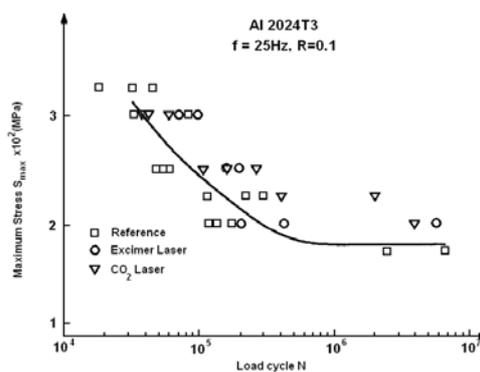
Fig. 2: *S-N* diagrams for fatigue tests of the reference and the treated Al 2024T3 specimens. (The data points for the treated specimens have been displaced downwards, relative to Fig. 1, by an amount
