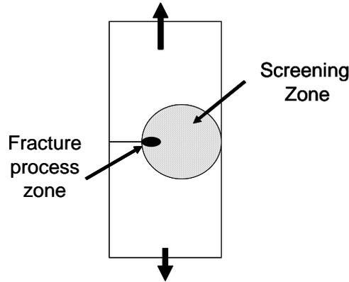
Figure 4: Schematic presentation of double volume approach with fracture process zone and screening zone.
