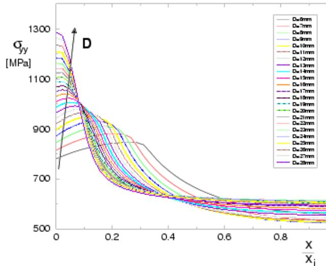
Figure 1: Evolution of Stress distribution with size (SENB specimen).
