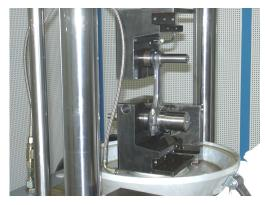
maintenance of the wanted strength; in the first phase the load linearly grows from time 0 to the value of with speed, for instance, equal around to 1KNw/ s. Subsequently, for an equal period to about 60 s, the load starts to oscillate around the value with an equal ampleness to 8KNw; the machine tries to stabilize the frequency for the value of the imposed load.
